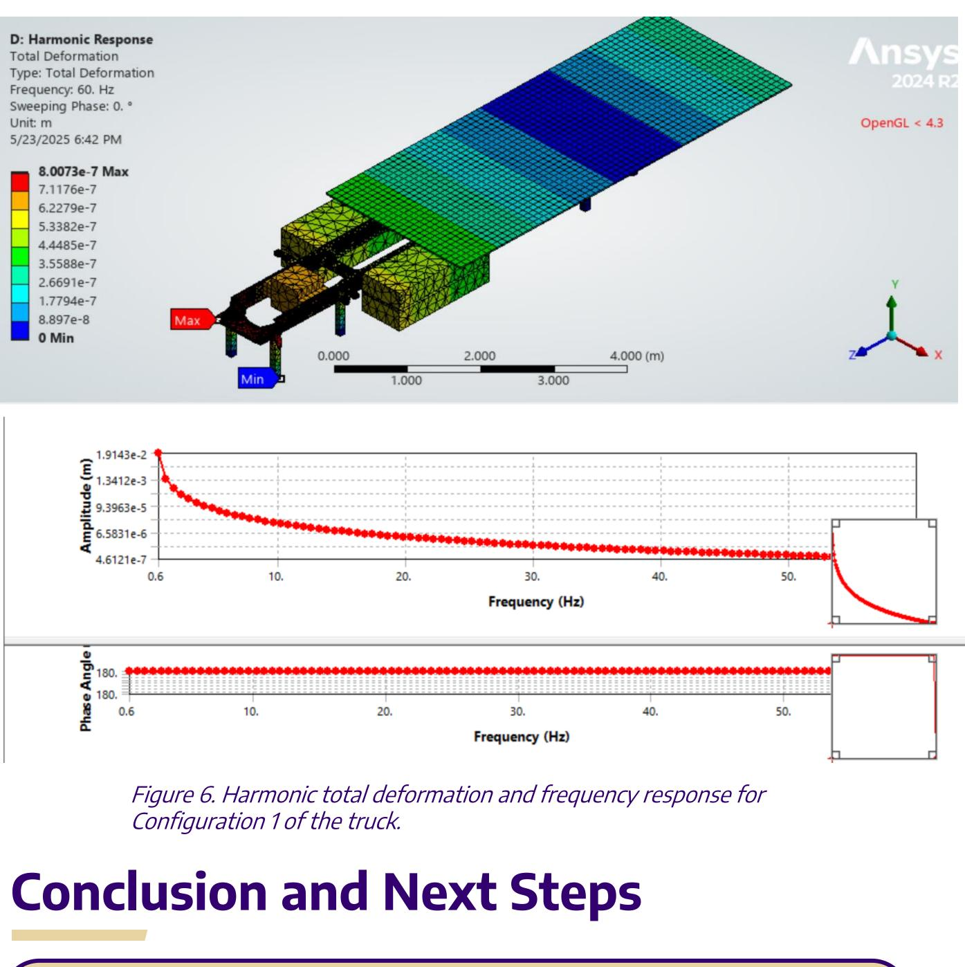
The Simulink and FEA models are expected to facilitate the finalization of design choices regarding performance, component mounting positions and controls systems. According to the tests, none of the configurations will resonate with the frequencies imparted by the road. Configuration 1 experiences the least amount of deformation. Future projects include HV cable routing, HIL test bench, and digital twin tuning.
