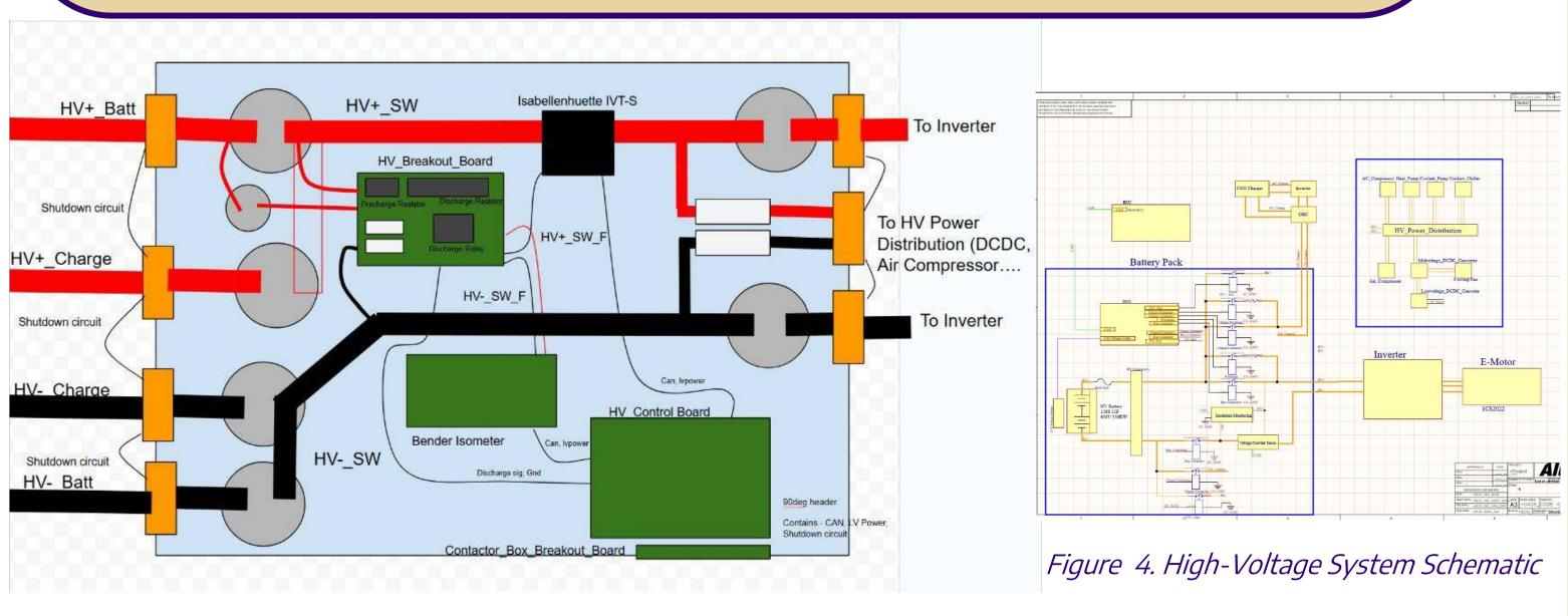
Figure 3. High-Voltage Contactor Box Layout
