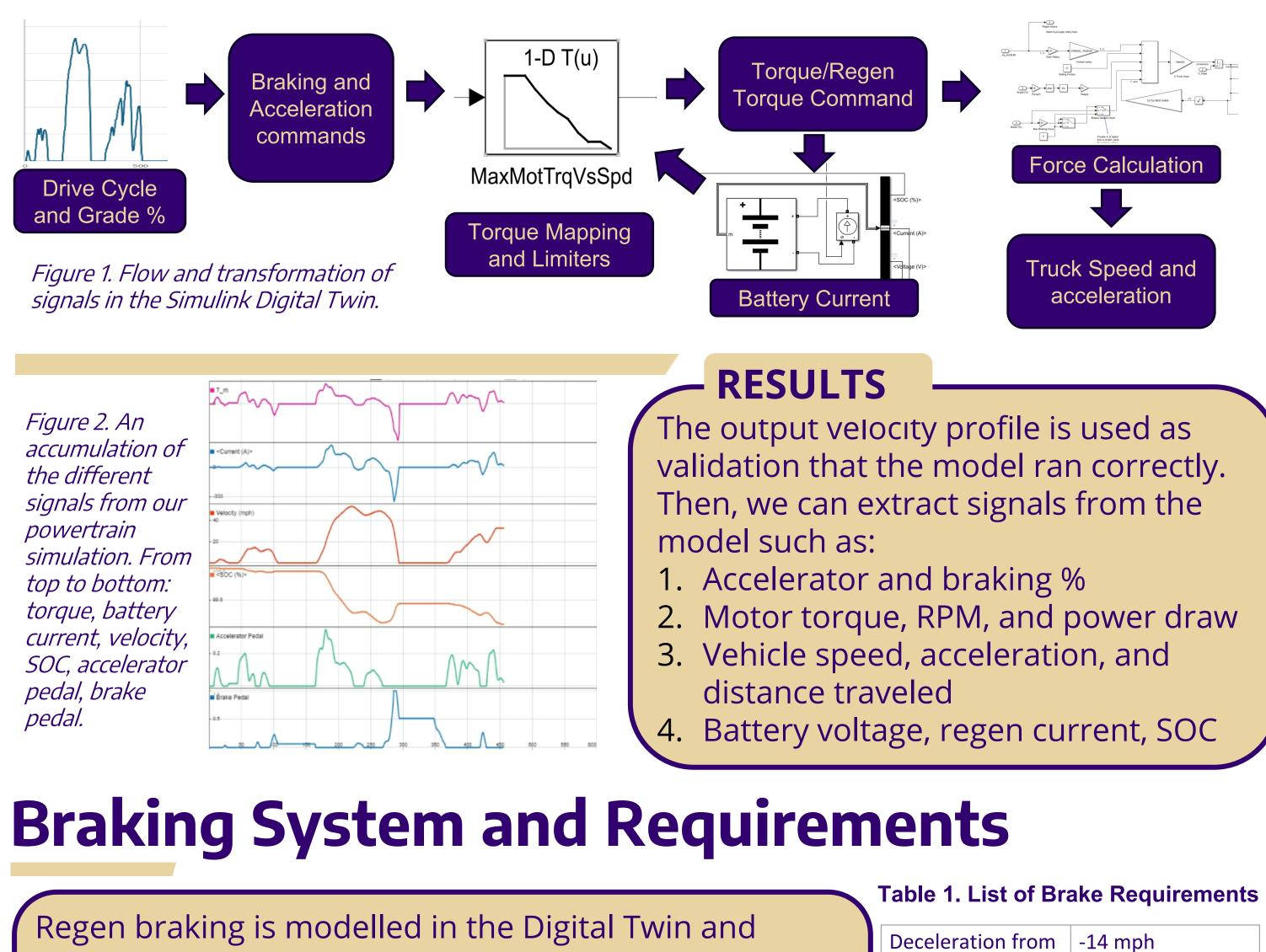
represents the motor behavior. The old brakes will be reused since we are choosing an e-motor, and a Bendix E-compressor will regulate the air pressure. Air braking will only be applied if regen does not meet required deceleration or if brake % passes a certain threshold.
